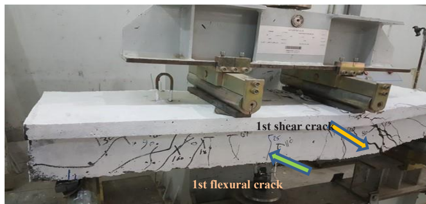
Fig 7. BG-max specimen after test
