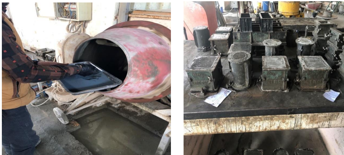
Fig 3. depicts the casting and specimens for the (RPC)
