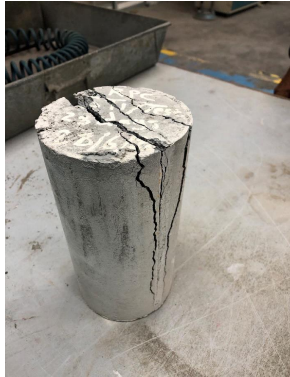
Fig 10. concrete failure behavior under tensile and crack pattern of (RPC)
