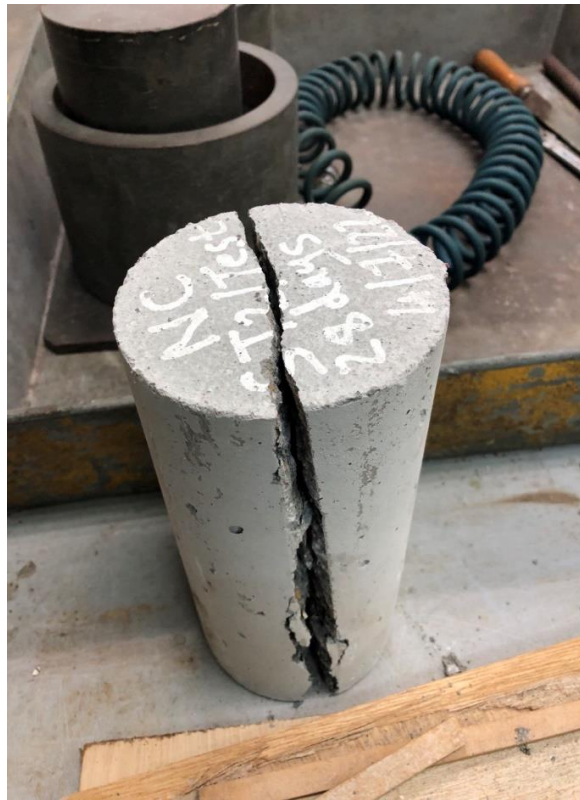
Figure 8. Concrete failure behavior under tensile and crack pattern of (NC)
