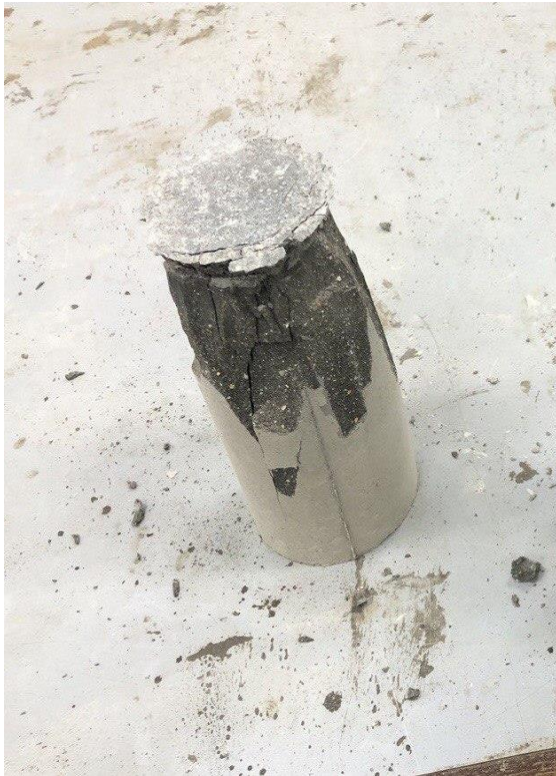
Fig 9. concrete failure behavior under compression and crack pattern of (RPC)
