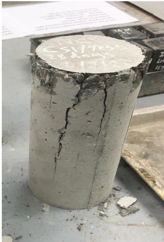
Figure 7. concrete failure behavior under compression and crack pattern of (NC)
