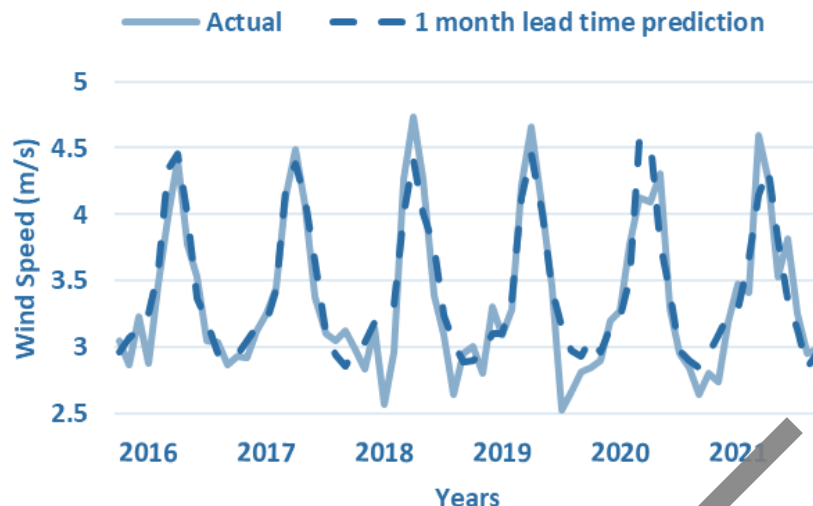
Fig. 2. Displays the watched and anticipated time arrangement of wind speed throughout the verification period utilizing the RF model.
