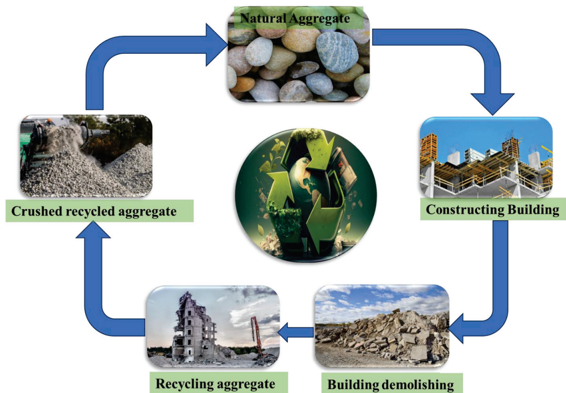
Fig. 1. The Process of producing RAs.
