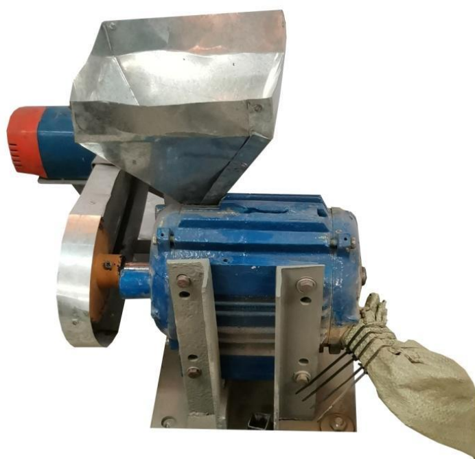
Fig. 2. Laboratory installation of a rotary centrifugal unit
