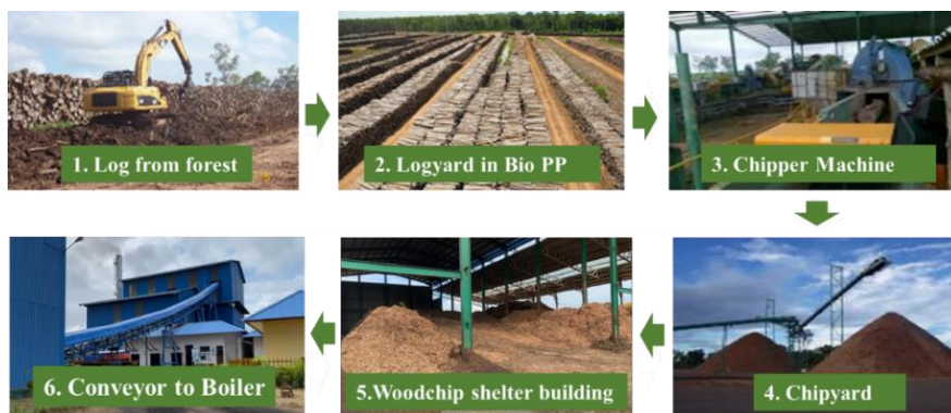
Fig. 3. Process flow diagram of feedstock from log to woodchip.
