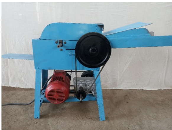
Fig. 3. A compact shredder with a convenient transmission channel.
