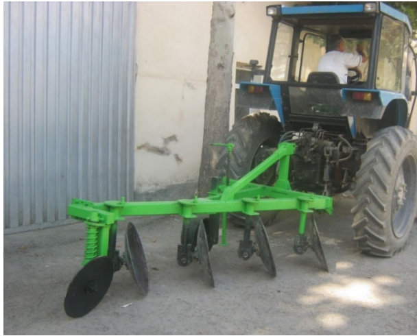
Fig. 2. View of disc plow mounted on tractor.
