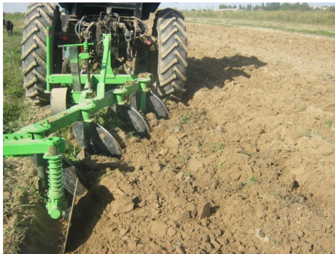
Fig. 3. View of the disk plow in operation.
