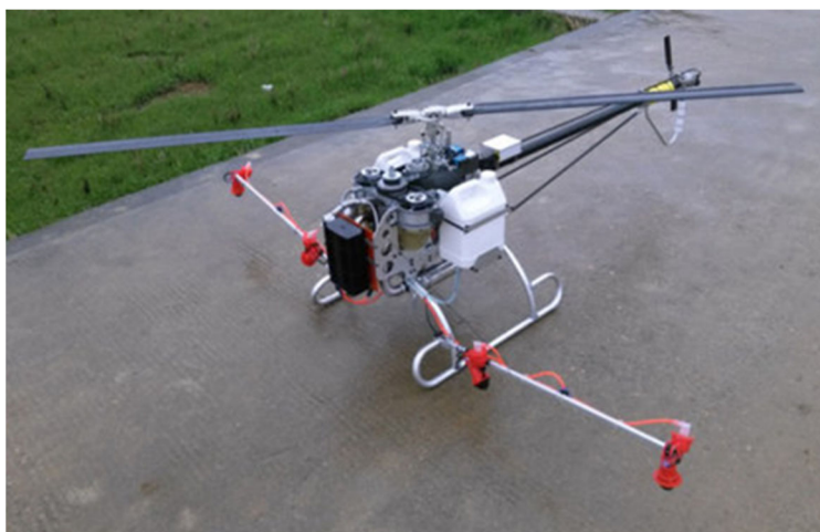
Fig. 1. CE-20 crop dusting unmanned helicopter.
