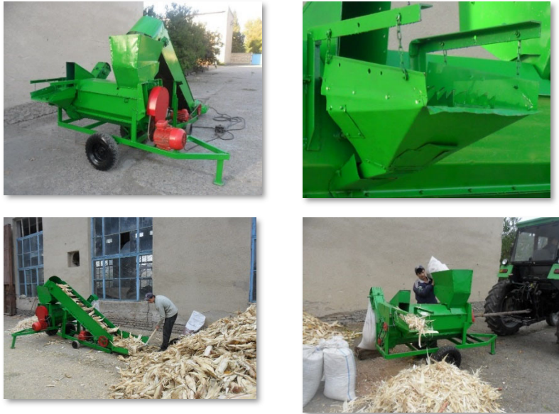
Fig. 3. Experimental sample and testing process of sieve of the corn-thresher machine.
