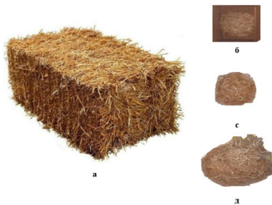
Fig. 1. Compressed wheat straw and its fractional composition: a) compressed wheat straw bale; b) length up to 30 mm, c) length between 30-50 mm d) fractions with length more than 50 mm.
