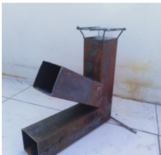
Fig. 4. Air input-port, firewood-port and fire output-port
