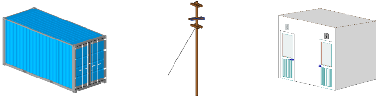
Fig. 2. Elements for organizing a construction site.
