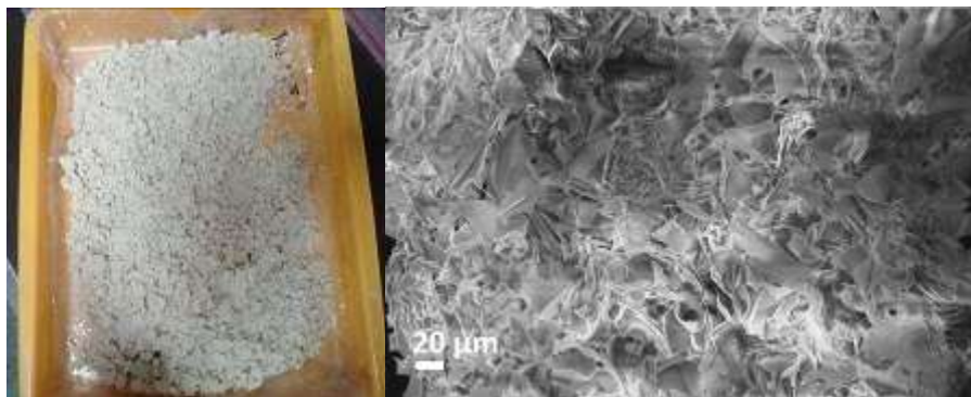
Fig. 1. Morphology of cellulose fibers from agar solid residue after alkali treatment and bleaching: (left) macro appearance and (right) under SEM observation 500 x magnification.
