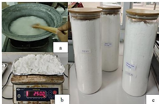
Fig. 2. Salt Samples: a) Recrystallization the salt, b) Weighing the salt before it is formulated with knife clams ( Solen spp.), c) Salt resulting from evaporation
