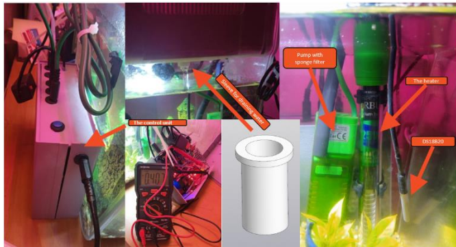
Fig. 2. Explanations on the location of key elements in the design of a home aquapon installation
