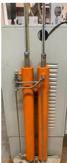
Fig. 4. Double-acting hydraulic cylinders on a test bench for testing throttle flow dividers/adders
