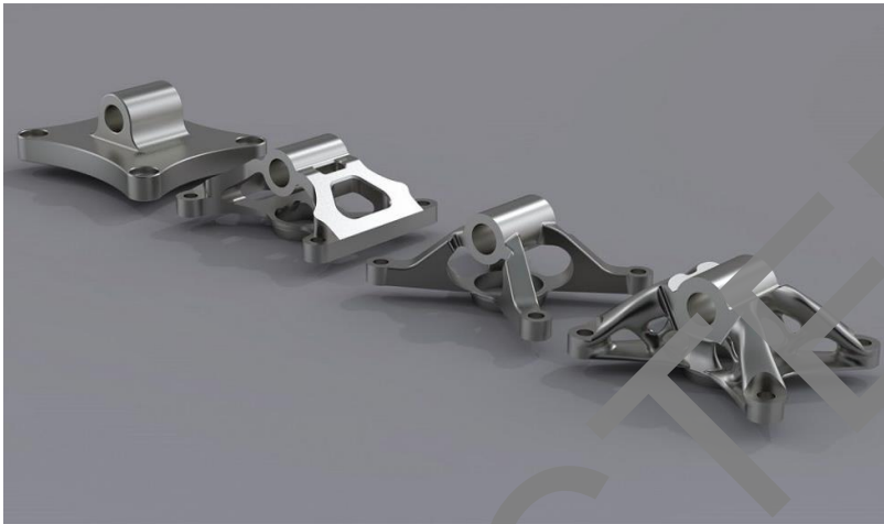
Fig. 2. Generated unconventional structure [10]
