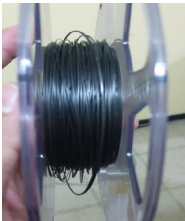
Fig. 1. Extrusion product: filament of nanocomposite PLA-nanographite.
