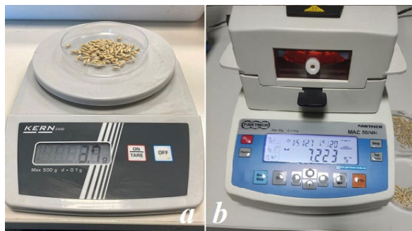
Fig. 2. Measuring instruments: a) digital weighing; b) moisture analyzer.
