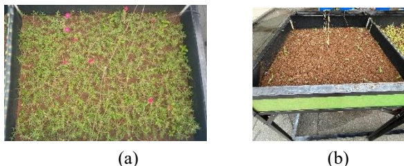
Fig. 2. Green roof planted with Portulaca grandiflora (a) and unvegetated green roof (b).
