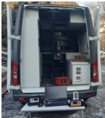
Fig. 1. Mobile laboratory for monitoring environmental safety and technical condition of transport facilities, transport infrastructure and industry.
