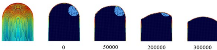
Figure 3: Evaporation sequences of a simulated Al-Fe tip with a high field precipitate.
