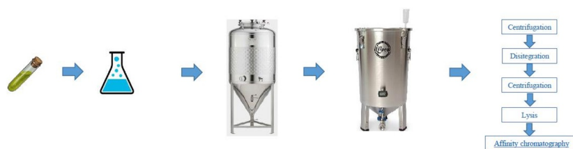
Fig.3. Fermentation and harvesting of E.coli lemo to produce hGH.
