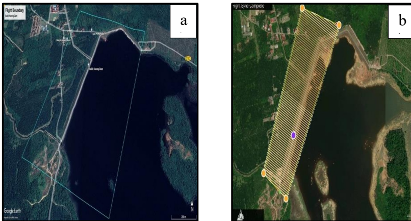
Figure 4. Flight design of UAV survey. (a) Flight boundary and (b) parallel-axis flight lines of Bukit Kwong dam for UAV operation that includes dam, downstream and upstream area. Boundary mission was constructed in Google Earth in KML format and exported into UAV.
