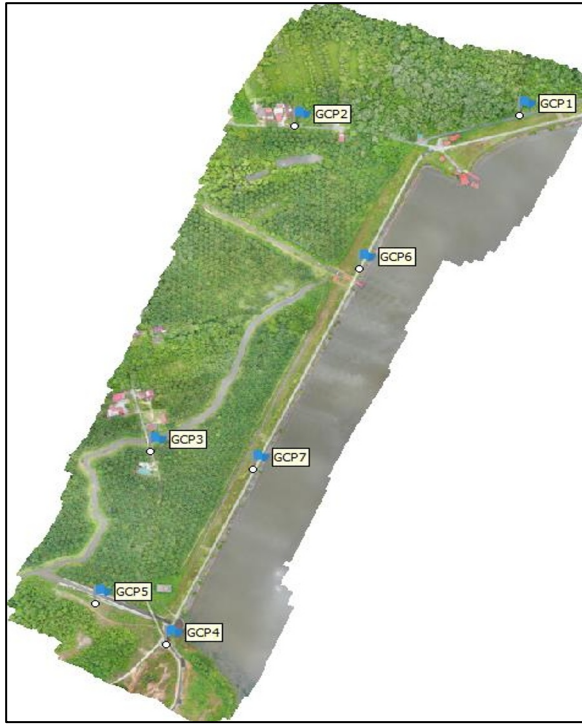
Figure 8. The distribution of seven ground control points in study area. Two GCPs (GCP 6 and 7) located at centre on embankment crest, while five GCPs located at upstream (GCP1, GCP 2), downstream (GCP 4 and 5) and at upper edge (GCP3) of study area.
