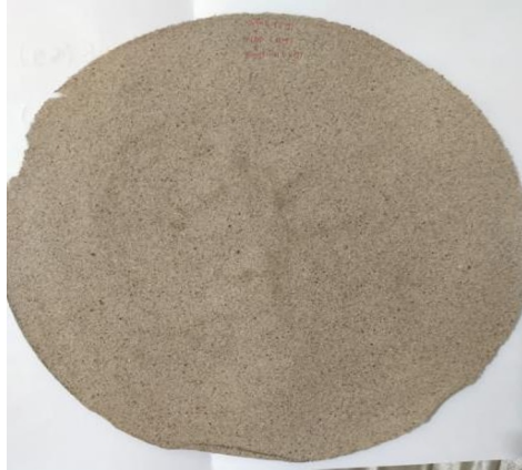
Fig. 1. The paper prepared from carton box (5g), WBP (4g) and Eggshell (4g)
