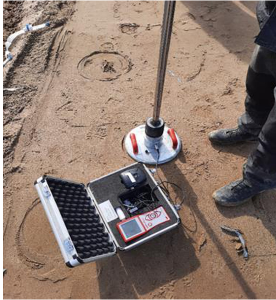
Fig. 2. Determination of the elastic modulus by installing a dynamic loading HMP LFG.
