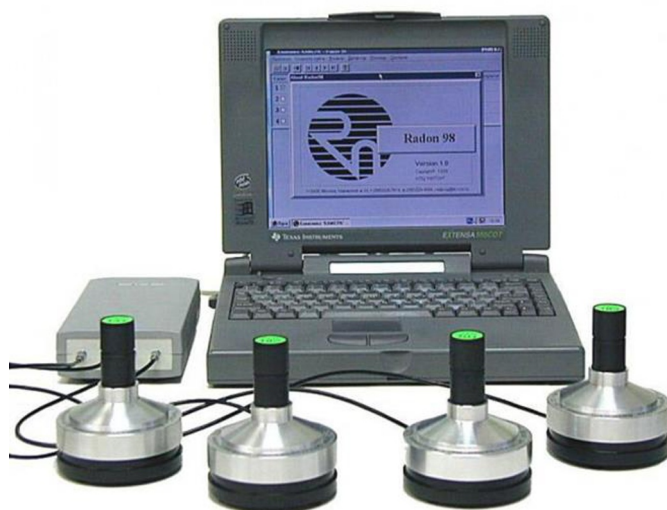
Fig. 1. Measuring complex for radon monitoring "CAMERA-01"
