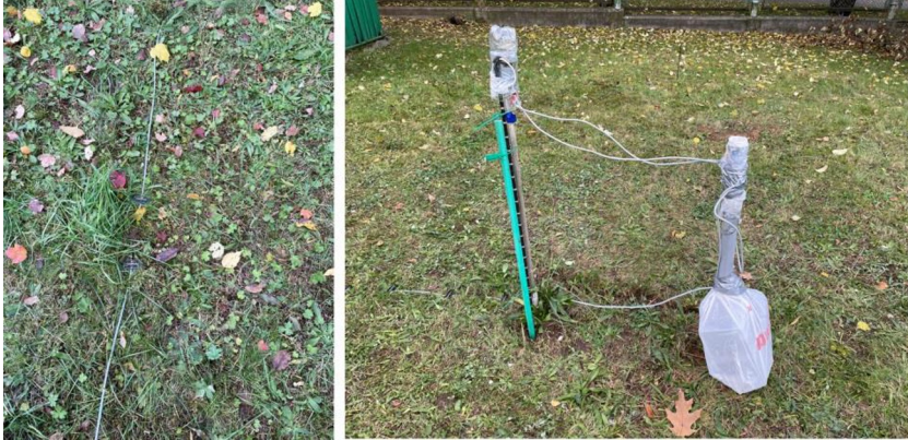
Fig. 3. Thermal sensors placed vertically and on the ground surface on the meteorological site.
