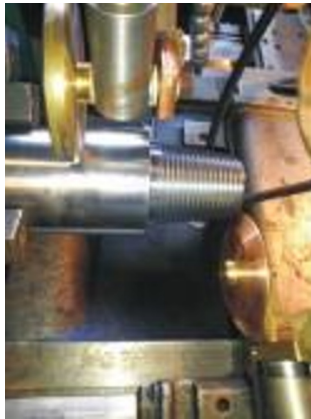
Fig. 2. Electromechanical locking thread finishing
