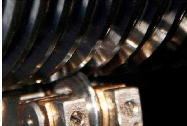
Fig. 3. The thread running-in with rollers
