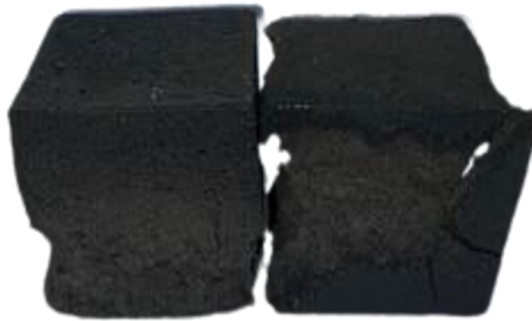
Fig. 3. The appearance of the specimens after the compressive strength test
