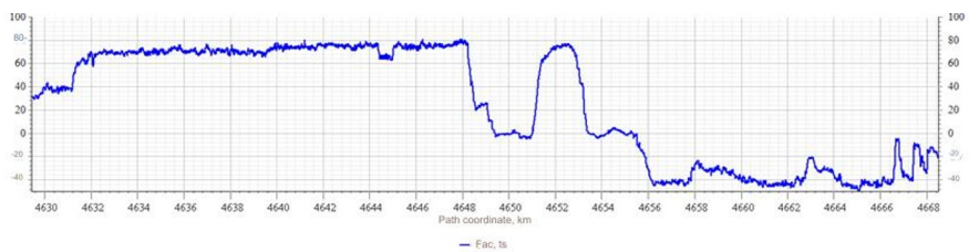
a) force on the automatic coupler of the laboratory car, tf
