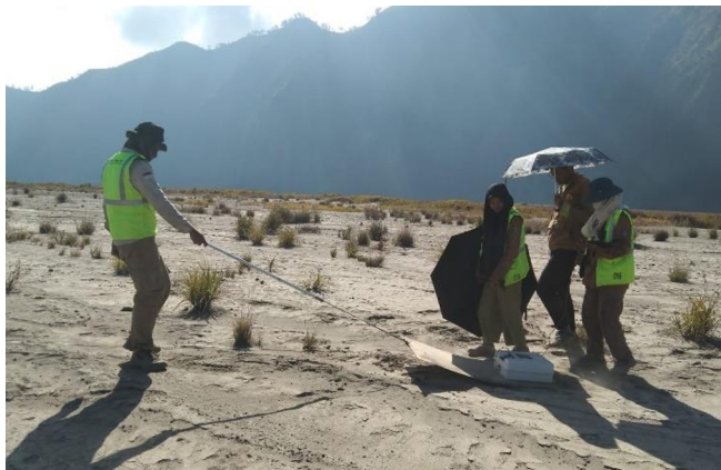
Fig. 4. GPR acquisition process (a) drone-based (b) ground-based
