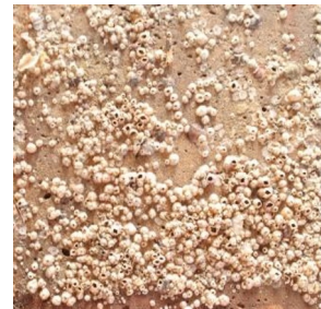
Fig. 2. Concrete Cube Covered with Barnacles at Tidal Zone Under Suramadu Bridge, Indonesia
