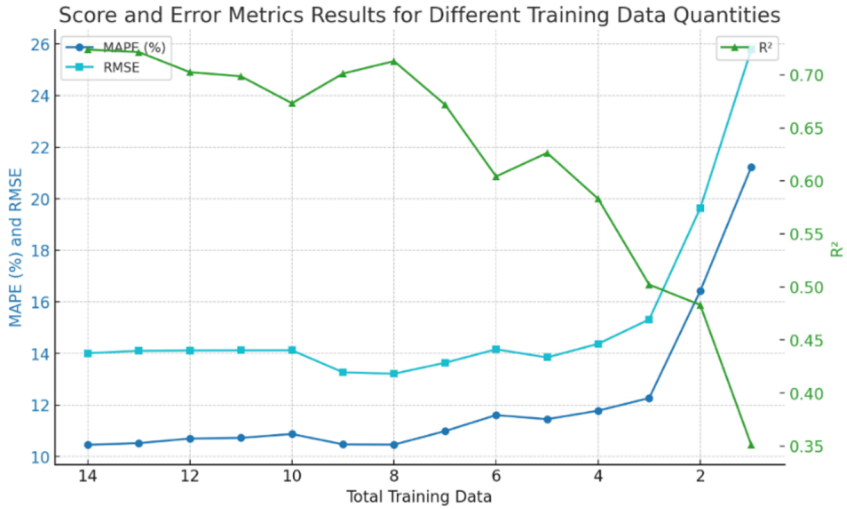
Fig.10. Comparison of Error Values and Correlation (R 2 ) Across Different Training Data Quantities
