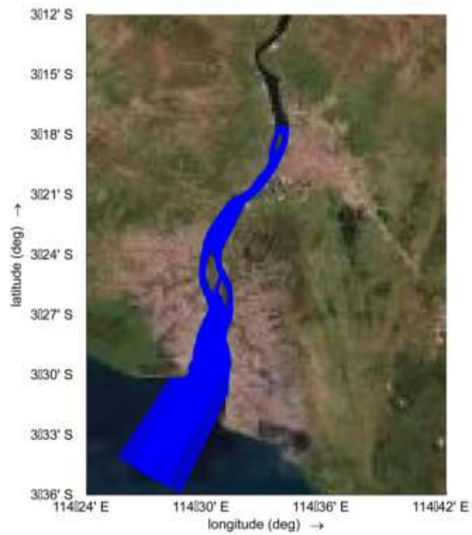
Fig. 5. Details of the model grid design, focusing on the Barito River Estuary with smaller grid sizes to capture finer spatial resolution.
