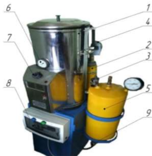
Figure 1. Small-volume biogas plant: 1 - reactor; 2 - small gas holder; 3 - burner; 4 - electro-contact manometer; 5 - gas holder; 6 - bimetallic thermometer; 7 - temperature regulator; 8 - programmer OVEN PR 110; 9 - safety valve.
