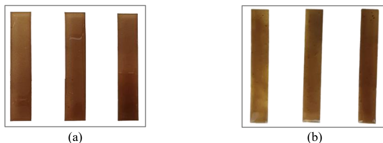
Fig. 2. (a) Biopolymer CB (Pectin-based biopolymer from coffee husk) and (b) biopolymer CCB (the combination)
