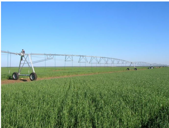
Fig. 3. CASCADe sprinkler machine (installation)
