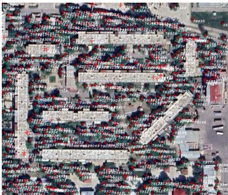
Fig. 2. True-color satellite map of Yashnabod district, showing individual tree locations marked in red, with unique ID numbers assigned by the AI model.
