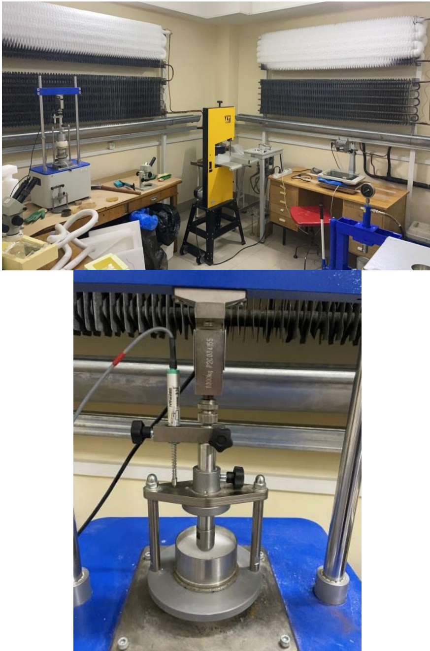
Fig.1. Cold laboratory of the geography department of MSU. Sealing device and installation of ASIS with the ball stamp device.
