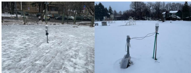
Fig. 1. Observing system for ground, snow and near-Earth air temperature at the MSU meteorological observatory site.
