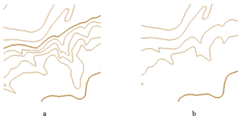
Fig. 9. Contours with a section height of 10 meters before generalization (a) and after automatic selection of isolines taking into account a section height of 20 meters (b). The isolines are partially removed. On large-scale topographic maps, relief is shown with a section of 2, 5 or 10 meters, on small-scale maps – 20, 50, 100 meters and more.
