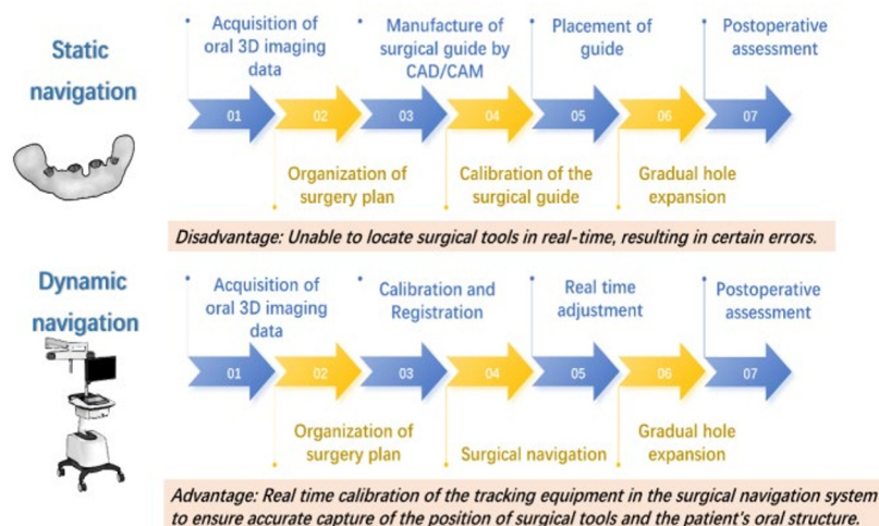
Figure 2. The operation procedure of static and dynamic navigation.
