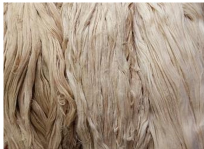
Fig. 2. Color variation in fibers due to moisture content.
