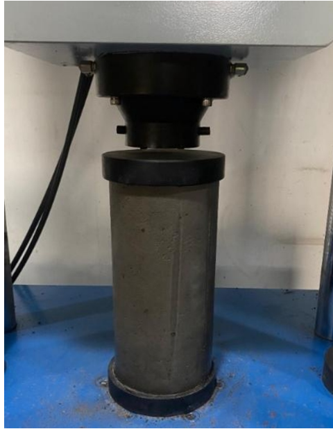
Fig. 3. Compressive Strength Testing of Cylindrical Concrete Specimen Using Digital Compression Machine.
