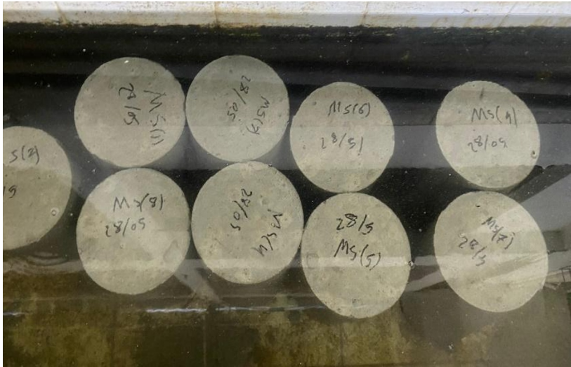
Fig. 2. Concrete Specimen Curing Setup Under Laboratory Conditions.
