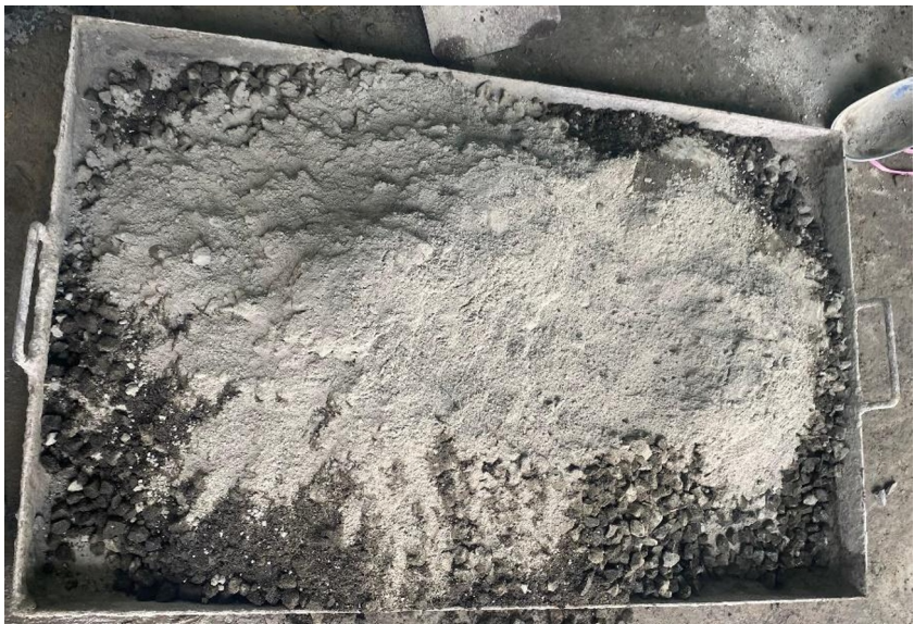
Fig. 1. Manual Preparation of Concrete Mix Components.
