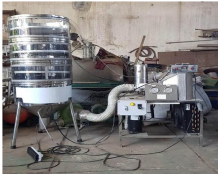
Fig. 1. Dehumidified cold air drying technology for drying marungga leaves
