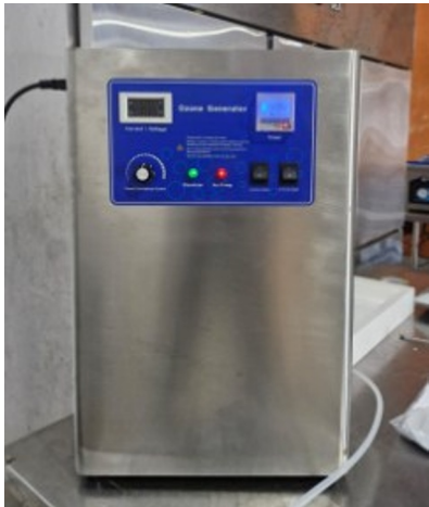
Fig 3. Ozone generator unit (20 g/h)
