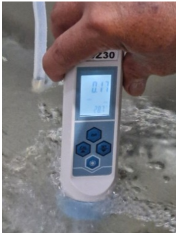
Fig. 4. DOZ-30 ozone analyzer for dissolved ozone measurement
