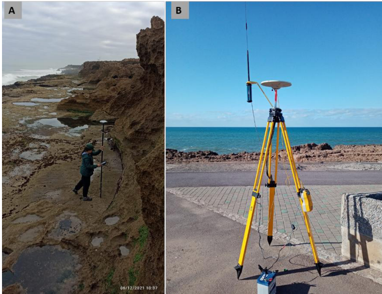
Fig. 2. Topographic data acquisition setup: (A) Field survey using the GPS-RTK rover in Sidi Moussa cliff; (B) Fixed base station for differential correction
