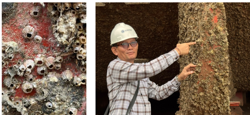
Fig. 1. Biofouling attack on ship hull: (a) barnacle dominated, and (b) barnacles, calcareous deposit, and soft fouling on ship's rudder
